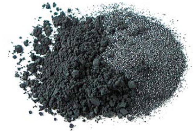
Technical ceramics - boron carbide (B 4 C), D 50 = 10 μm
