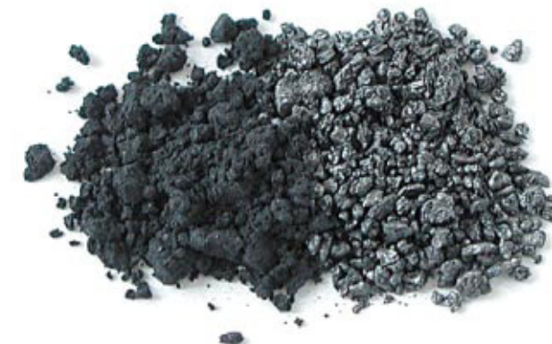
carbone – graphite synthétique (C), D 50 = 6 μm
